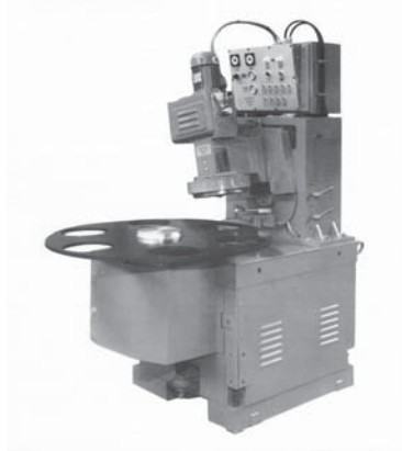
A machine for making pottery saucers. This one produces 14 pieces a minute.
